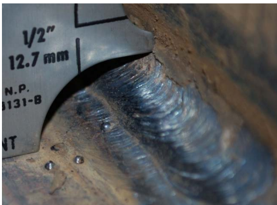
A 3/16" 7018 can potentially produce a 5/16" weld size with one pass and 1/2" with 3 passes.
