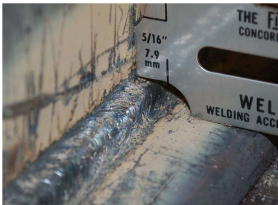
A 3/16" 7018 can potentially produce a 5/16" weld size with one pass and 1/2" with 3 passes.
